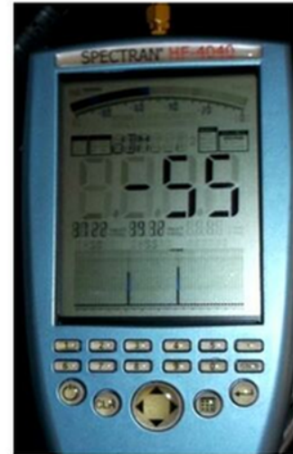
Figure 3. Another typical Spectran HF-4040 reading, 3722 MHz at -58dbm and 3932 MHz at -55dbm. The power level seems to be determined by the building structure over the target's head – i.e., a residential roof or a multi-floor building.
