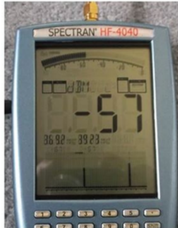
Figure 2. Another typical Spectran HF-4040 reading, 3692 MHz at -67dbm and 3923 MHz at -57 dbm.
